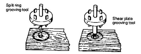
Figure 5-30. - Tools used for grooving wood for timber connectors.
