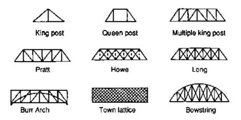
Figure 2-13<sup>---</sup> Typical truss configurations for timber bridges.
