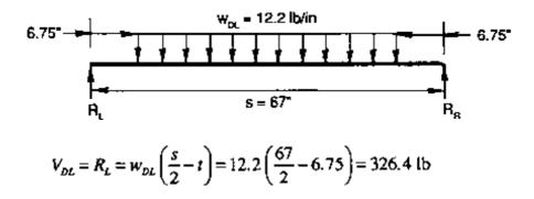
Live load vertical shear is computed at the lesser distance of 3t or s/4 from the support:
