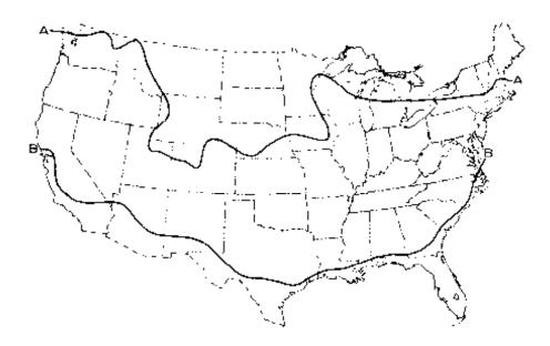
Figure 13-8. - (A) The northern limit of recorded damage done by subterranean termites in the United States. (B) The northern limit of damage done by drywood termites.
