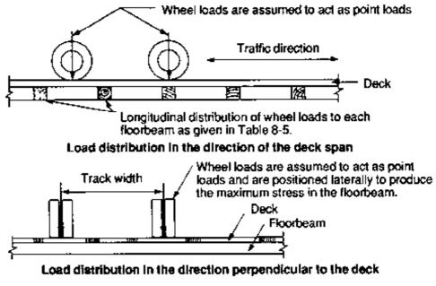
Figure 8-17. - Wheel load distribution to transverse floorbeams that directly support a longitudinal timber deck.
