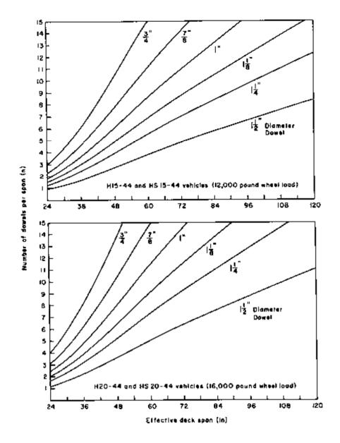
Figure 7-22. - Number of dowels required for each effective span of a doweled glulam deck.
