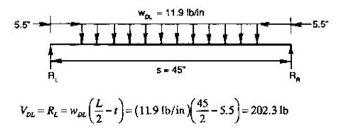
Live load vertical shear is computed at the lesser of 3t or s/4 from the support:
