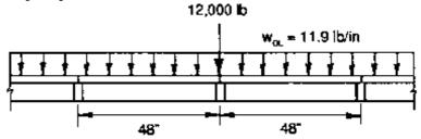
$$R_{DL} = (48 \text{ in.})(w_{DL}) = (48 \text{ in.})(11.9 \text{ lb/in}) = 571.2 \text{ lb}$$
