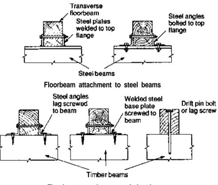
Floorbeam attachment to timber beams
