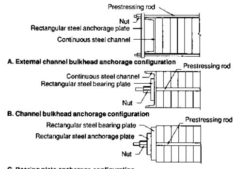
C. Bearing plate anchorage configuration
