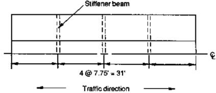
The size and stiffness of an individual stiffener beam must be sufficient to provide a minimum E'I value of 80,000 k-in<sup>2</sup>. A glulam stiffener will be used because of the improved dimensional stability of glulam compared to sawn timber. Selecting a combination symbol No. 2 stiffener, 5-1/8 inches wide and 6 inches deep:
