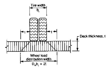
Figure 8-11. - Wheel load distribution width for continuous longitudinal nail-laminated lumber decks.
