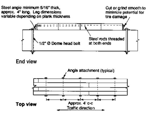
Figure 11-28. - Attachment detail for lumber running planks using threaded rods and steel angle brackets.
