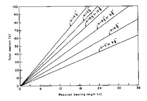
Figure 7-10.—Approximate adjusted minimum bearing length for glulam beams based on an allowable compression perpendicular to grain,  $F_{e\perp}$ , of 344.5 lb/in<sup>2</sup> ( $F_{e\perp}$  =  $F_{e\perp x}C_M$  = 650 lb/in<sup>2</sup> (0.53)).
