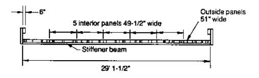
Section properties are computed for the smaller 49.5-inch panel width:
