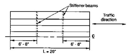
The size and stiffness of the stiffener beam must be sufficient to provide a minimum EI value of 80,000 k-in<sup>2</sup>. Selecting a combination symbol No. 2 glulam stiffener, 6-3/4 inches wide and 4-1/2 inches deep (dry-use conditions may be used for glulam stiffener beams if they are protected by a watertight deck):
