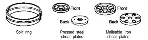
Figure 5-26. - Types of timber connectors.
