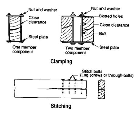
Figure 14-13. - Typical configurations for clamping and stitching timber members.
