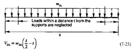
where  $V_{DL}$  = dead load vertical shear (lb).
