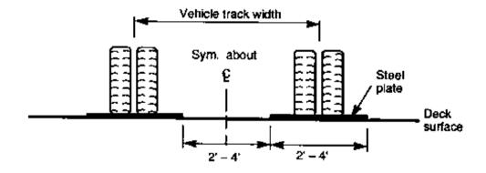
Figure 11-22. - Typical steel plate wearing surface cross section.
