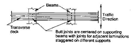
Figure 7-36. - Joint placement for transverse nail-laminated lumber decks.
