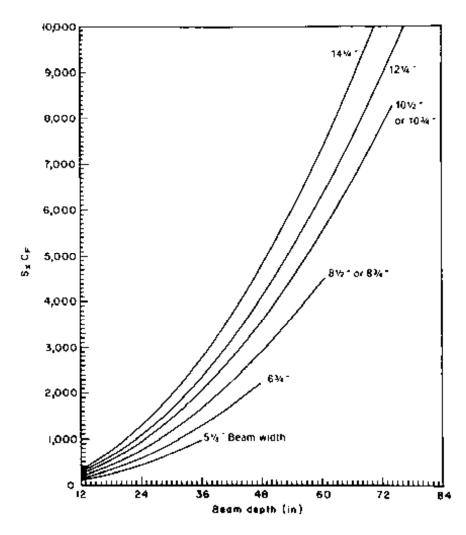
Figure 7-9. - Approximate adjusted section modulus  $(S_x C_F)$  versus beam depth for standard glulam beam widths.
