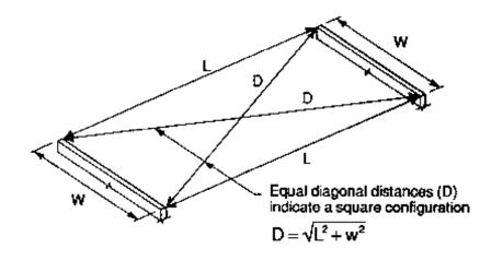
Figure 12-10. -- Verifying squareness and alignment of substructures by measurement of diagonals.
