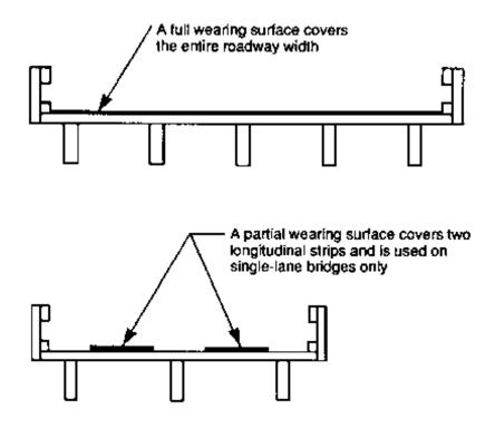
Figure 11-1. - General wearing surface configurations.
