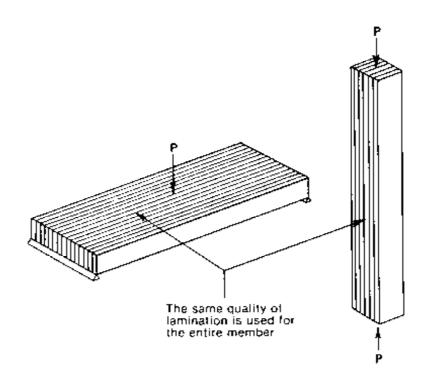
Figure 3-34.- Glulam axial combinations are intended primarily for applications where loads are applied parallel to the wide face of the laminations. The same quality of lumber lamination is used for the entire member.
