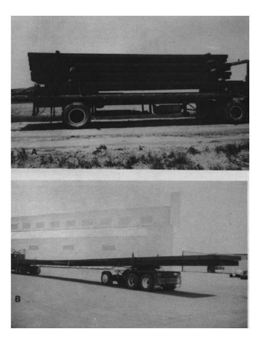
Figure 12-5. - Truck transportation of timber bridge components. (A) Short members, such as these nail-laminated lumber deck panels, can be transported on a flatbed truck (photo courtesy of Wheeler Consolidated, Inc.). (B) Long glulam beams require specialized vehicles such as this log truck and dolly (photo courtesy of Western Wood Structures, Inc.).
