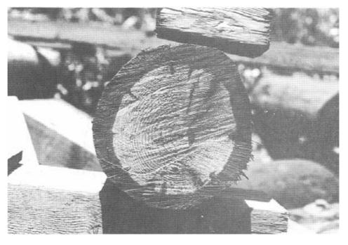
Figure 4-1.- Cross section of a coastal Douglas-fir pile treated with creosote. Note that the preservative treatment penetrates the outer sapwood ring but stops at the less permeable heartwood.
