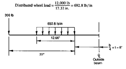
$V_{\mu} = (12.66 \text{ in.})(692.8 \text{ lb/in}) = 8,771 \text{ lb}$
