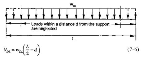
where  $V_{DL}$  = vertical dead load shear at a distance *d* from the support (lb) and
