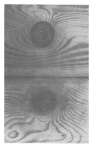
Figure 3-18.- Types of knots. (Top) encased knot and (bottom) intergrown knot.
