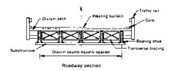
Figure 7-2. - Typical glulam beam bridge configuration.
