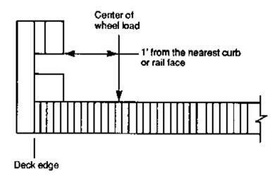
The maximum spacing of prestressing rods is obtained using the curve in Figure 9-18, based on the distance from the outside deck edge to the center of the wheel load. The spacing of the first rod from the deck end is generally equal to one-half the center-to-center spacing.
