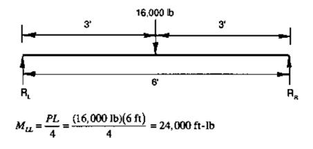
Allowable bending stress is computed using the beam size factor,  $C_F$ Consideration of lateral stability is not required because the floorbeams are continuously supported by the deck:
