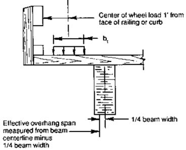
Deck stress in bending and horizontal shear must be within allowable values previously determined.
