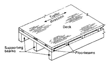
Longitudinal deck supported on transverse floorbeams
