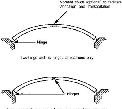
Three-hinge arch is hinged at reactions and at the arch apex.
