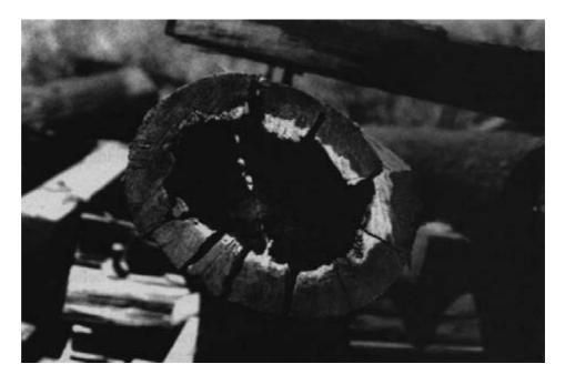
Figure 13-43. - Internal decay in a timber pile where it was drift-pinned to the cap. Before the breakage of the outside shell, caused by cap removal, the pile showed little exterior sign of the interior decay.
