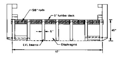
Figure 9-7. - Drawing of a stress-laminated T-bridge cross section.
