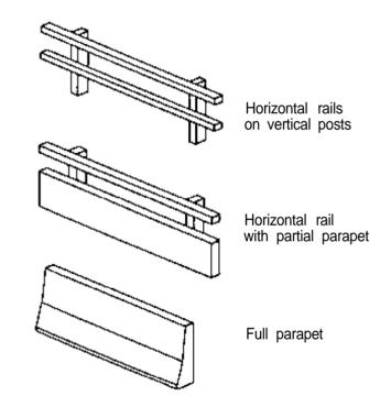
Figure 10-2. - Typical configurations for vehicular railing used on timber bridges.
