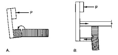
Figure 10-10. - Two types of potential timber bridge damage resulting from rail impact loads. (A) Separation in a longitudinal glulam or nail-laminated lumber deck from tension perpendicular to the laminations. (B) Beam damage resulting from forces transferred by a post brace.
