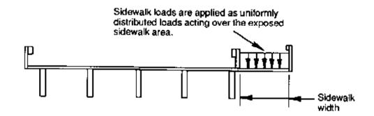
Figure 6-26. - Application of side walk loads.
