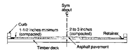
Figure 11-4. - Typical asphalt pavement wearing surface cross section.
