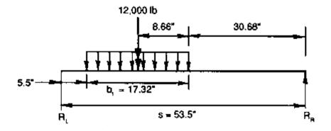
$$V_{LL} = R_L = \frac{(12,000 \text{ lb})(8.66 \text{ in.} + 30.68 \text{ in.})}{53.5 \text{ in.}} = 8,824 \text{ lb}$$
