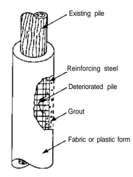
Figure 14-12. - Reinforced concrete jacket for pile augmentation.
