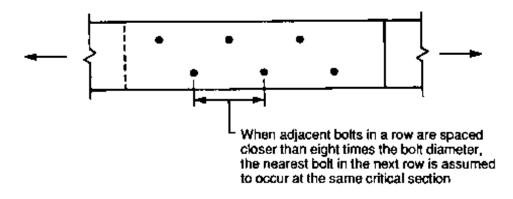
Figure 5-20. - Critical section for determining net area for staggered bolts loaded parallel to grain.
