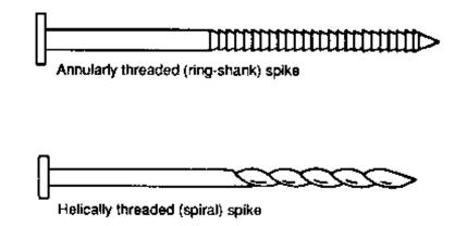
Figure 11-17. - Types of spikes used for attaching lumber wearing surfaces.
