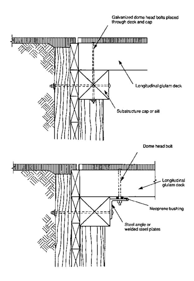
Figure 8-7. - Typical bearing configurations for longitudinal glulam decks.
