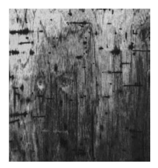
Figure 13-11. - Damage by Ambrosia beetles in green wood. The galleries are free of residue and the surrounding wood is darkly stained.
