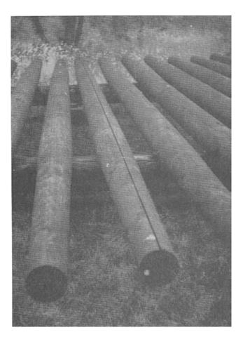
Figure 4-7.—Kerting large wood members, such as this pole, can reduce the potential for checking in service.
