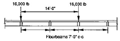
For the minimum 14-foot axle spacing, maximum longitudinal distribution is one axle load per floorbeam.
