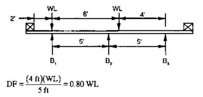
For outside beams, the distribution factor is the same as that obtained for moment, DF = 1.0 WL/beam.
