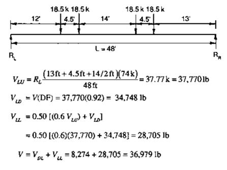
Stress in horizontal shear is computed by Equation 7-7:
