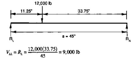
$$V = V_{pL} + V_{1L} = 202.3 + 9,000 = 9,202.3 \text{ lb}$$
