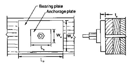
Figure 9-19. - Bearing-plate anchorage configuration.
