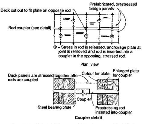
Figure 9-12. - Method of joining two prefabricated, prestressed longitudinal stresslaminated bridge panels.
