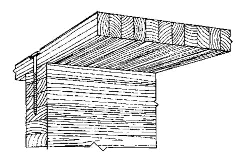
Figure 7-25. - Lag screw connection for attaching glulam decks to glulam beams.
