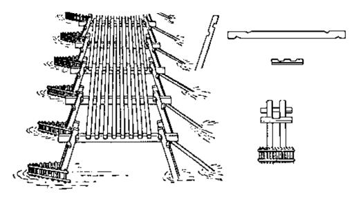
Figure 1-2.–Caesar's Bridge according to Palladio (photo courtesy of the American Society of Civil Engineers: © 1976. Used by permission.)
