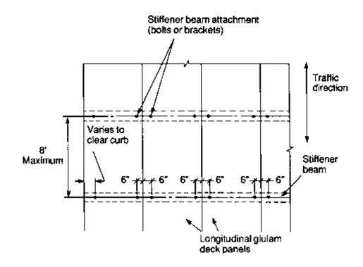
Figure 8-6. - Stiffener-beam attachment for longitudinal glulam decks.
