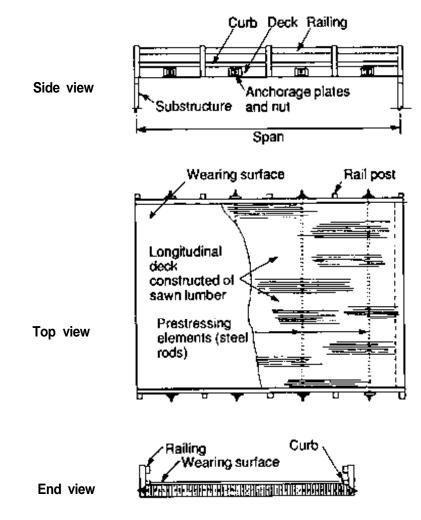
Figure 9-1. - Typical configuration for a longitudinal stress-laminated lumber deck bridge.
