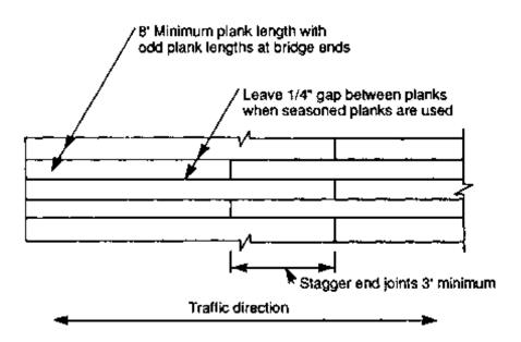
Figure 11-14. - Typical plank layout for lumber wearing surfaces.
