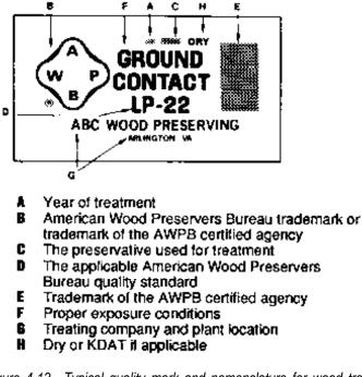
Figure 4-13.- Typical quality mark and nomenclature for wood treated in accordance with AWPB quality standards (courtesy of the American Wood Preservers Bureau). Used by permission.
