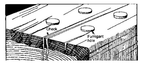
Figure 14-8. - Treating holes for fumigants in horizontal members should be placed on both sides of checks or splits, and be bored to within 1-1/2 to 2 inches of the bottom of the member.
