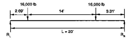
$$V_{WL} = R_L = \frac{(16,000 \text{ lb})(3.31 \text{ ft} + 17.31 \text{ ft})}{20 \text{ ft}} = 16,496 \text{ lb}$$
