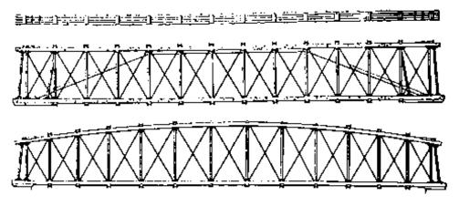
Figure 1-17.- Pratt truss as patented in 1844 (photo courtesy of the American Society of Civil Engineers; <sup>©</sup> 1976. Used by permission).
