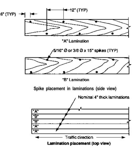
Figure 8-14. - Spike placement for longitudinal nail-laminated deck panels constructed of nominal 4-inch-thick lumber laminations.
