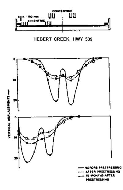
Figure 15-46. - Load test results at the Hebert Creek Bridge, before and after transverse prestressing was applied.
