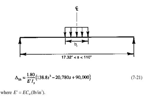
When the effective deck span is greater than or equal to 110 inches  $(s \ge 110)$ , maximum live load deflection is obtained when both wheel loads are centered on the span and is computed as follows:
