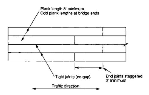
Figure 11-27. - Typical plank layout for a lumber running plank wearing surface.
