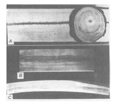
Figure 3-19.-(A) Eccentric growth about the pith in a cross section containing compression wood. The dark area in the lower third of the cross section is compression wood. (B) Axial tension break caused by excessive longitudinal shrinkage of compression wood. (C) Warp caused by excessive longitudinal shrinkage of compression wood.
