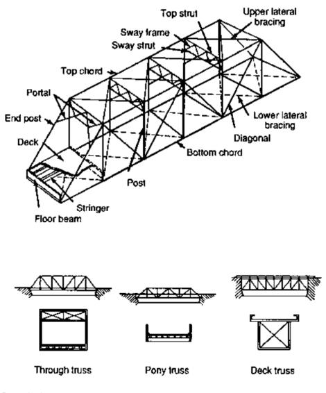
Figure 2-12.—Truss bridge nomenclature and classifications.
