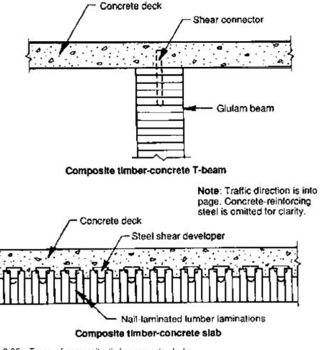
Figure 2-25.- Types of composite timber-concrete decks.
