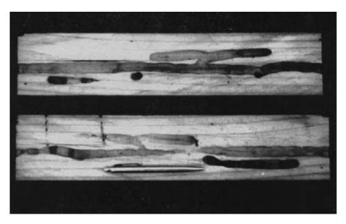
Figure 13-14 - Carpenter bee damage in wood. The bees bore long tunnels along the grain to lay their eggs (photo courtesy of USDA Forest Service, Forest Sciences Laboratory, Gulfport, Mississippi).
