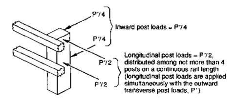
P' = the outward transverse post load applied to the post at each rail location (P, P/2, or P/3 from Figure 10-4)
