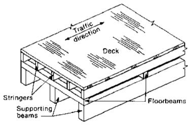
Transverse deck supported on longitudinal stringers, supported on transverse floorbeams
