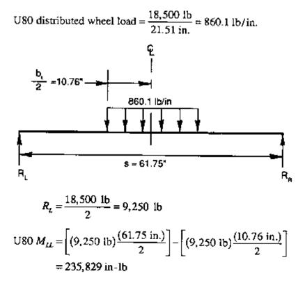
Dividing U80 moment by the allowable overload increase of 1.33 and comparing the value to H 20-44 moment indicates the controlling vehicle:
