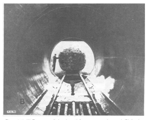
Figure 4-10.-(A) Treatment cylinders (retorts) for pressure-treating wood. (B) As vie wed from the inside of a cylinder, wood ready for treating is loaded on carts that are rolled into the cylinder on steel tracks.
