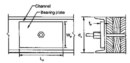
Figure 9-20. - Channel bulkhead anchorage configuration.
