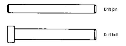
Figure 5-33. - Typical drift pin and drift bolt.
