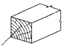
A pitch pocket is a well-defined opening that contains free resin. Pitch pockets are usually localized and do not extend far in the longitudinal direction.
