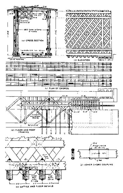
Figure 1-12.-Town's lattice truss patented in 1820 (photo courtesy of the American Society of Civil Engineers; © 1976. Used by permission).
