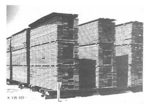
Figure 4-8.- Sawn lumber stacked for air drying. Note the thin wood strips or "stickers" placed between the lumber to permit free air circulation.
