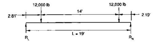
$$V_{LL} = R_L = \frac{(12,000 \text{ lb})(2.19 \text{ ft} + 16.19 \text{ ft})}{19 \text{ ft}} = 11,608 \text{ lb}$$
