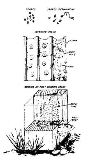
Figure 13-1. - The decay cycle (top to bottom). Fungi begin as minute spores that germinate and grow through the wood. Once enough energy has been obtained, the fungus produces a fruiting body and releases spores that spread and infect other wood.
