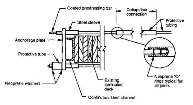
Figure 15-39. - Prestressing detail for rehabilitation of existing decks.
