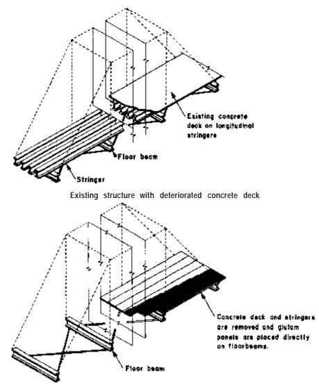
Deck replacement with longitudinal glulam panels
