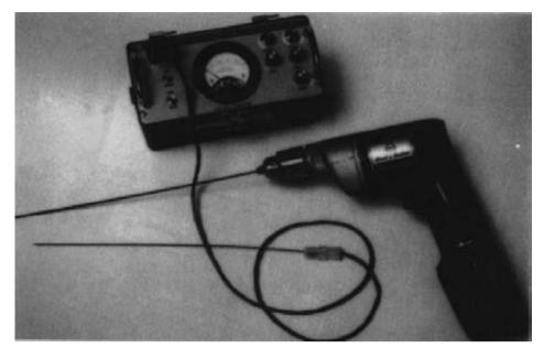
Figure 13-27. - A Shigometer and the drill and bit used to bore holes for insertion of the wire probe.
