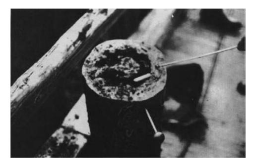
Figure 15-2. - Section of deteriorated pile removed from the structure.
