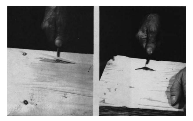
Figure 13-23. - The pick test for detecting earlywood decay. (Left) Sound wood pries out as long slivers. (Right) Decayed wood breaks abruptly across the grain without splintering.
