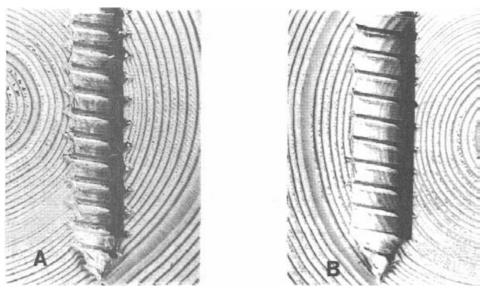
Figure 5-25. - (A) Clean-cut, deep penetration of thread made by a lag screw turned into a lead hole of proper size. (B) Shallow penetration of thread made by a lag screw turned into an oversized lead hole.
