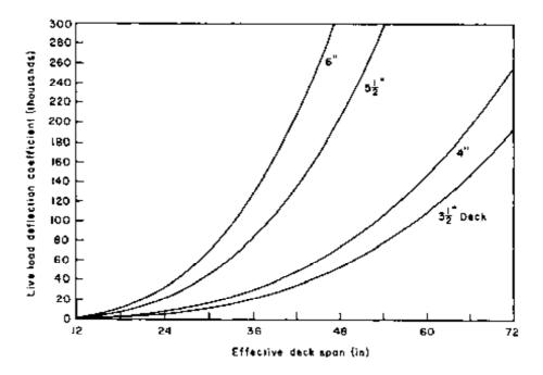
Figure 7-37. - Vehicle live load deflection coefficients for 12,000-pound wheel load(s) on a continuous, transverse nail-laminated lumber deck that is continuous over more than two spans. Divide the deflection coefficient by E' to obtain the deck deflection in inches.
