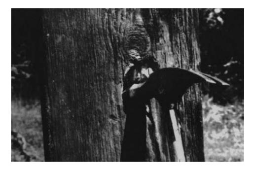
Figure 13-25. - A decay pocket near the wood surface is detected by sounding with a hammer.
