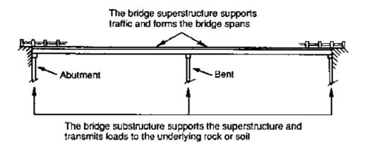
Figure 2-1.- Basic components of a timber bridge.
