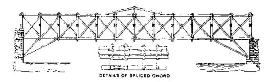
Figure 1-14.---Drawing of Long's truss bridge as patented in 1830 (photo courtesy of the American Society of Civil Engineers; <sup>©</sup> 1976. Used by permission).
