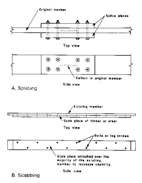
Figure 14-11. - Splicing and scabbing methods of member augmentation.
