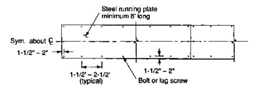
Figure 11-24. - Steel plate wearing surface attachment pattern using bolts or lag screws.
