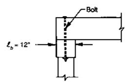
Bearing stress is checked for the bearing length,  $\ell_b$ , of 12 inches. From Table 16-8, the maximum reaction for one wheel line of an HS 20-44 truck on a 37-foot span is 26,920 pounds. The dead load reaction is computed using the bridge length of 38 feet:
