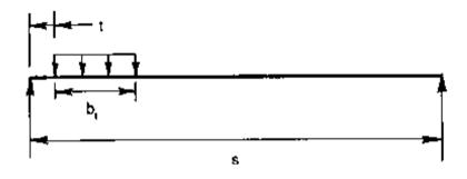
Applied stress in horizontal shear must be less than or equal to the allowable stress for the laminations, as computed by
