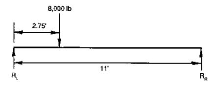
$$V_{LU} = R_L = \frac{(8,000 \text{ lb})(11 \text{ ft} - 2.75 \text{ ft})}{11 \text{ ft}} = 6,000 \text{ lb}$$
