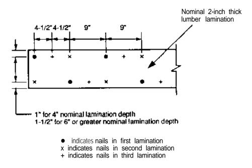
Figure 7-38. - Nail placement pattern for transverse nail-laminated lumber decks.
