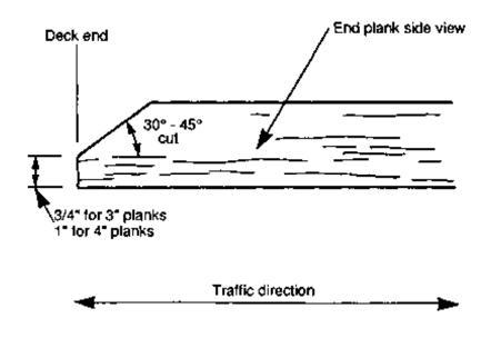
Figure 11-15. - Beveled end-plank configuration to minimize vehicle impact at bridge ends.
