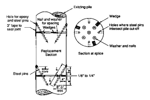
Figure 14-16. - Schematic diagram of pile posting.
