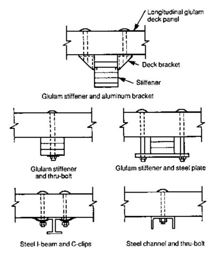
Figure 8-5. - Types of transverse stiffener-beam configurations for longitudinal glulam deck panels.
