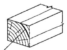
A shake is a separation or plane of weakness between growth increments that may extend a substantial distance in the longitudinal direction.
