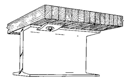
Figure 7-26. - C-clip for attaching glulam decks to steel beams.
