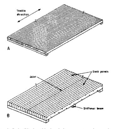
Figure 8-8. - Longitudinal nail-laminated lumber decks are constructed as continuous decks and as panelized decks. (A) In continuous decks, laminations are progressively nailed to adjacent laminations to form a continuous deck across the structure width. (B) For panelized decks, lumber is nail-laminated into panels that are interconnected with transverse stiffener beam(s).
