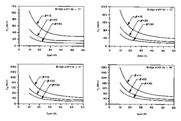
Graphs are based on a HS 20-44 vehicle with a maximum wheel load of 16,000 lb. For other wheel loads, multiply the graph value of  $V_r$  by the ratio of design wheel load to a 16,000-lb wheel load. Use interpolation and/or extrapolation for intermediate bridge widths and  $\beta_r$  values.
