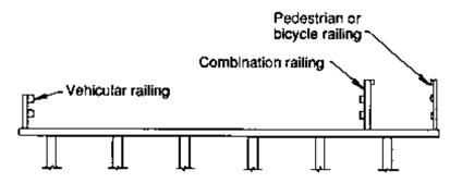
Figure 10-1. - Types of timber bridge railing.
