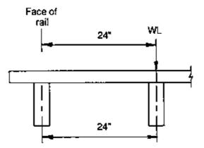
The moment DF to outside beams is technically zero; however, AASHTO requires that the DF to outside beams not be less than that to interior beams. The moment DF is therefore 0.50 WL/beam.
