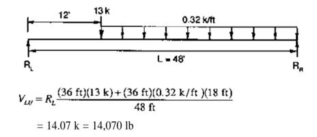
H 20-44 shear stress is computed for the controlling lane load:
