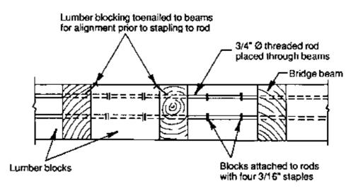
Figure 7-33. - Lumber block diaphragm configuration using steel rods and driven staples.
