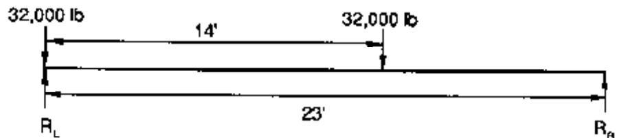
$$R_{MAX} = R_L = \frac{(32,000 \text{ lb})(23 \text{ ft} - 14 \text{ ft}) + (32,000 \text{ lb})(23 \text{ ft})}{23 \text{ ft}} = 44,522 \text{ lb}$$
