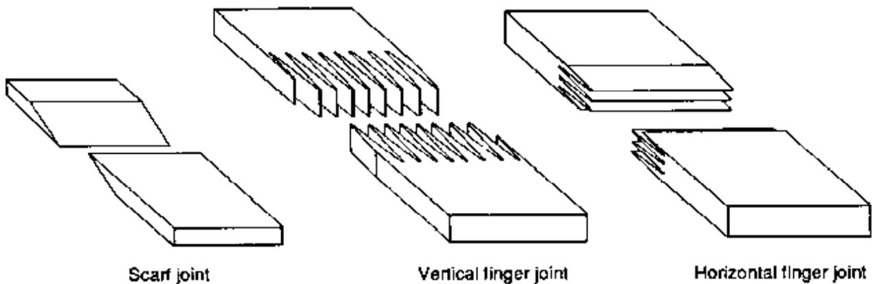
Figure 3-31.- Types of lamination end joints used in glulam.
