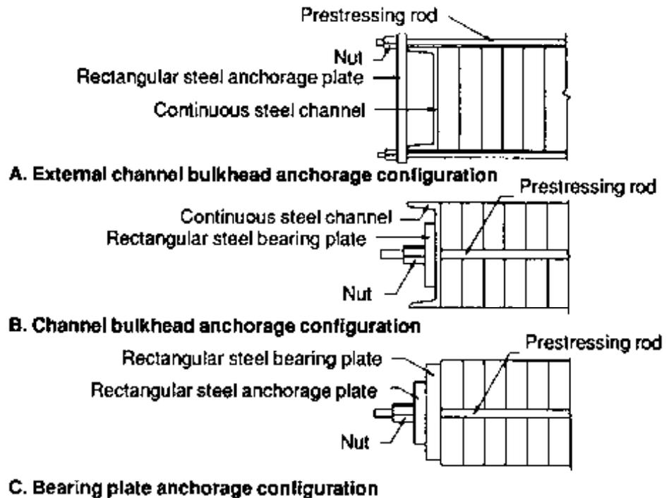
Figure 9-10. - Types of anchorages for steel prestressing rods.
