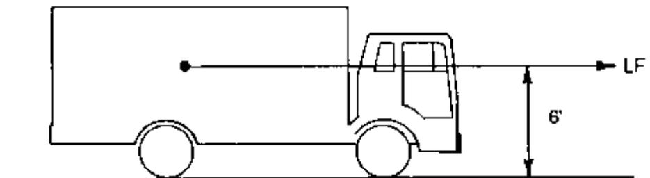
Figure 6-10. - Application of the vehicle longitudinal force.
