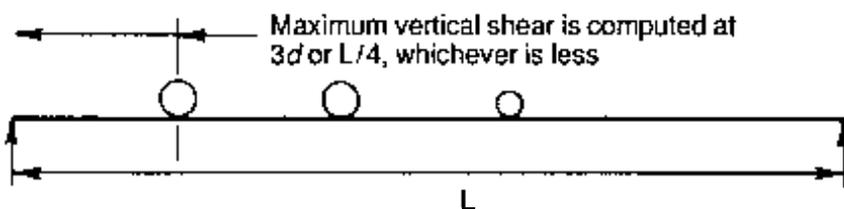
Figure 7-6. - Live load horizontal shear in timber beams is based on the maximum vertical shear occurring at a distance from the support equal to three times the beam depth ( $3d$ ), or the span quarter point ( $L/4$ ), whichever is less.
