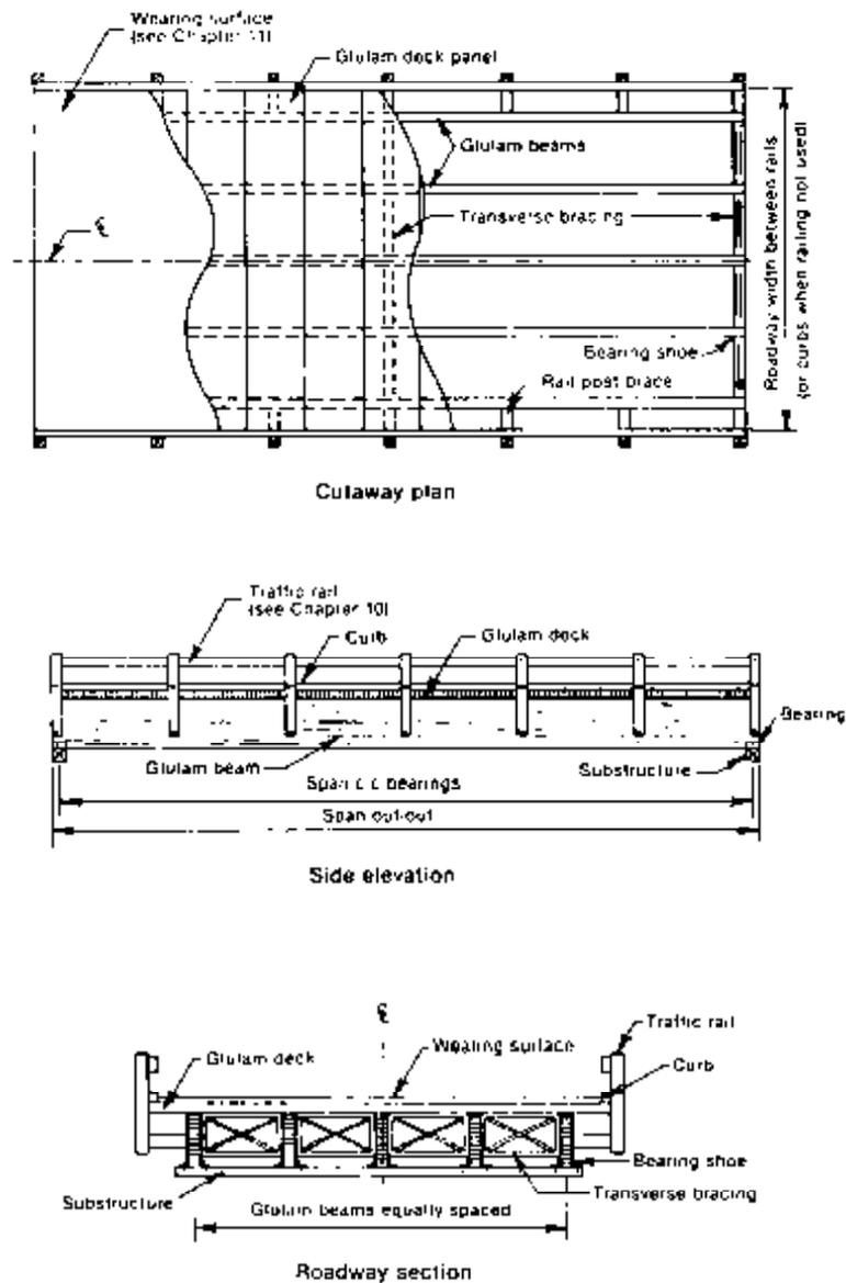
Figure 7-2. - Typical glulam beam bridge configuration.
