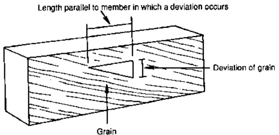
Figure 3-16.- Slope of grain measurement in wood members.
