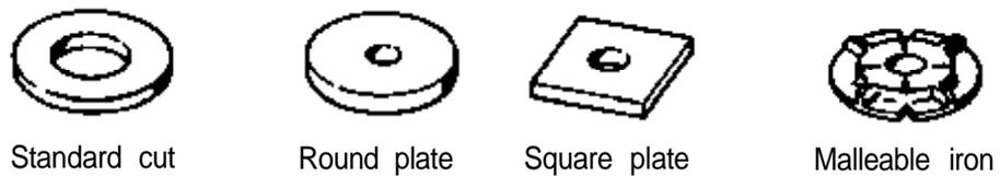
Figure 5-14. - Common washer types for timber connections.
