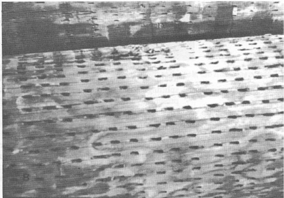
*Figure 4-5.-(A) The most common method of incising involves pressing small metal teeth into the wood surface. (B) The openings in the wood improve the penetration and retention of preservatives in many difficult- to-treat species.*
