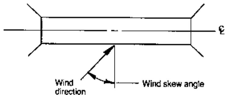
Figure 6-16. - Wind skew angle for substructure design.
