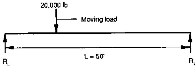
The tabulated stress for horizontal shear for a 24F-V2 beam is obtained from *AITC 117--Design*,
