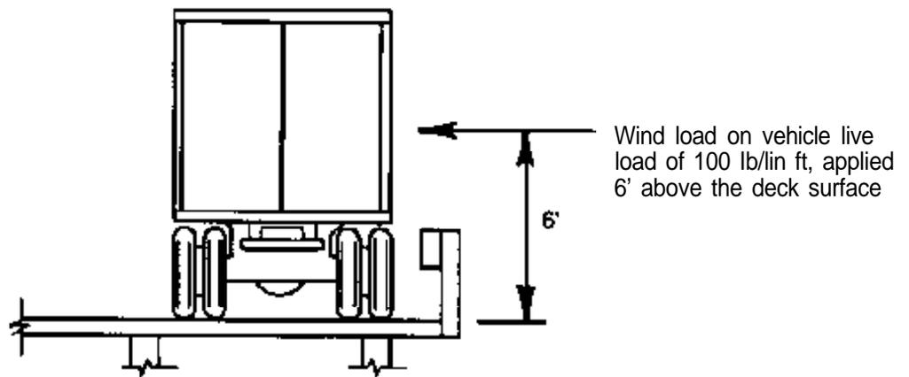
Figure 6-15. - Application of wind load acting on the vehicle live load.
