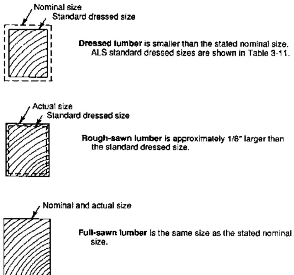
Figure 3-25.- Dressed, rough-sawn, and full-sawn lumber sizes.
