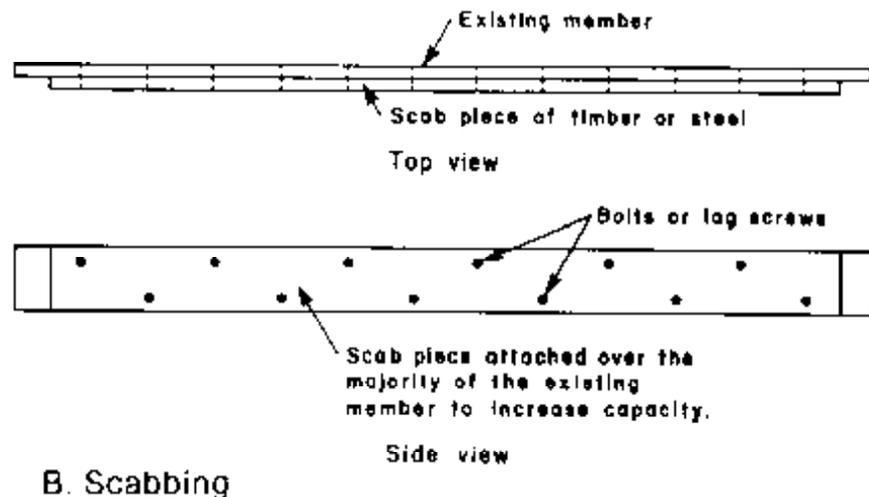
Figure 14-11. - Splicing and scabbing methods of member augmentation.
