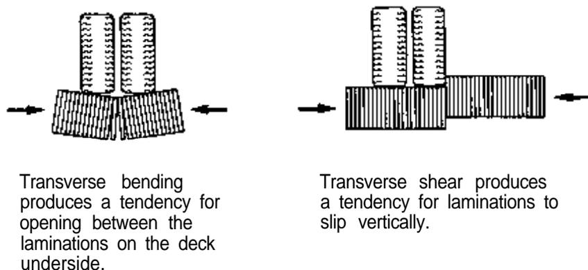
Figure 9-8. - Actions that tend to reduce the platelike behavior of a longitudinal stress-laminated bridge deck.
