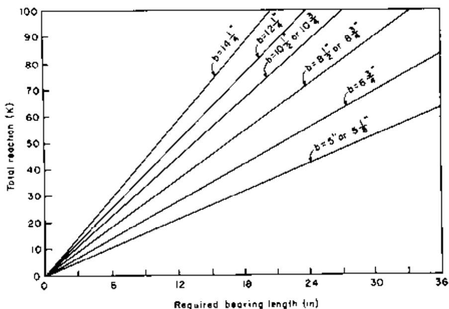
Figure 7-10.—Approximate adjusted minimum bearing length for glulam beams based on an allowable compression perpendicular to grain,  $F_{c\perp}'$ , of  $344.5 \text{ lb/in}^2$  ( $F_{c\perp}' = F_{c\perp} C_M = 650 \text{ lb/in}^2 (0.53)$ ).
