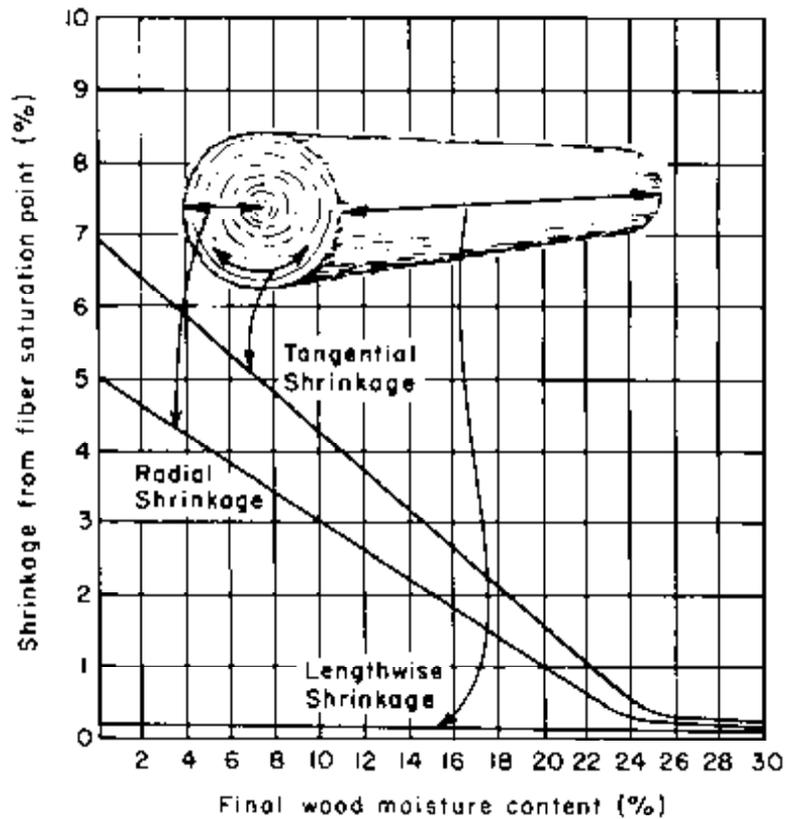
Figure 3-7.- Approximate wood shrinkage relationships below the fiber saturation point for the three orthotropic axes (adapted from the Canadian Wood Council<sup>13</sup>). Used by permission.
