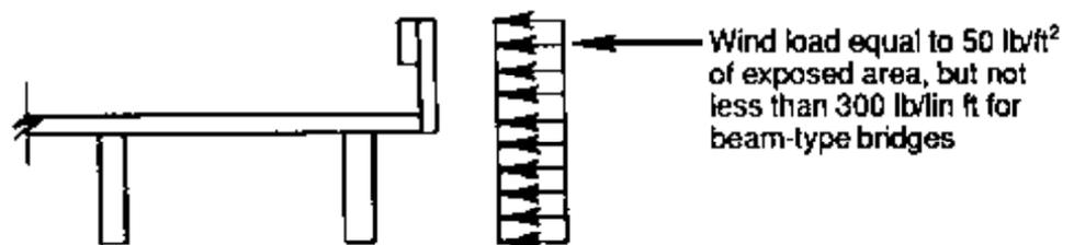
Figure 6-14. - Wind load applied to the bridge superstructure.
