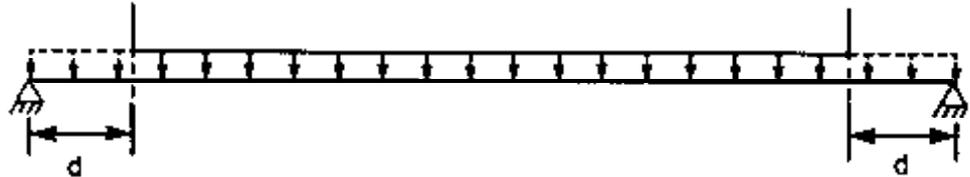
For stationary loads, such as dead load, the maximum vertical shear is computed at a distance d from the supports and all loads occurring within a distance d from the supports are neglected
