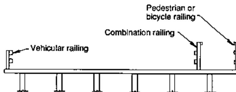
Figure 10-1. - Types of timber bridge railing.
