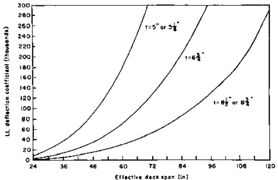
Figure 7-19. - Vehicle live load deflection coefficients for 12,000-pound wheel load(s) on a transverse, noninterconnected glulam deck that is continuous over more than two spans. Divide the deflection coefficient by  $E'$  to obtain the deck deflection in inches.
