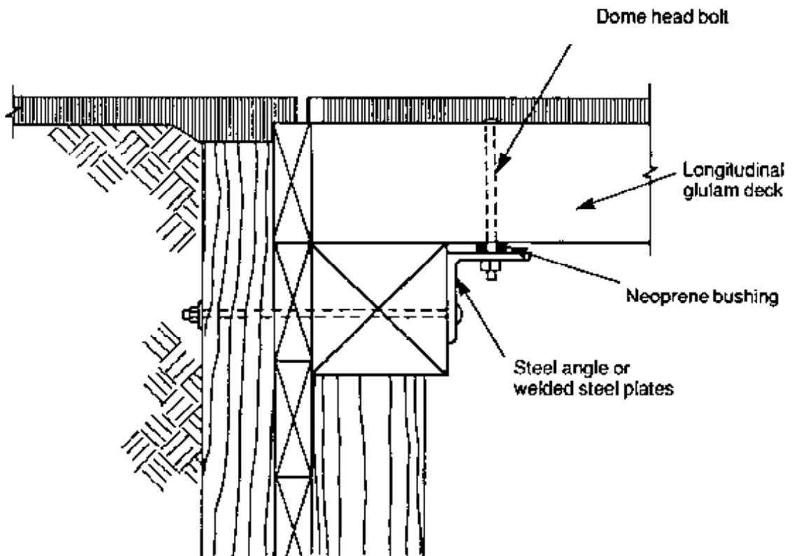
Figure 8-7. - Typical bearing configurations for longitudinal glulam decks.
