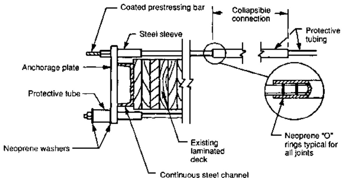
Figure 15-39. - Prestressing detail for rehabilitation of existing decks.
