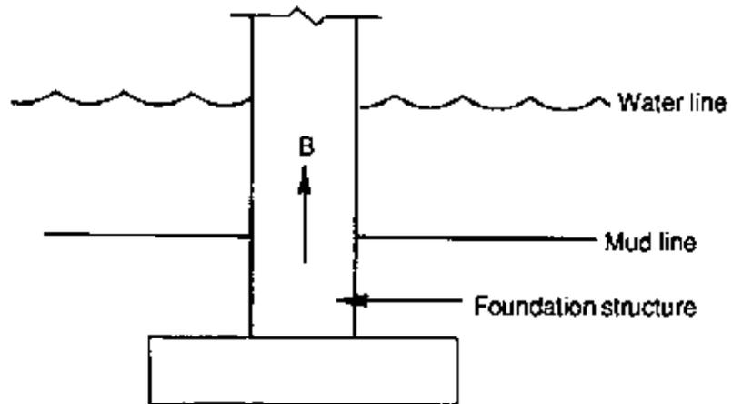
The buoyancy force (B) is an upward vertical force equal in magnitude to the volume of the structure below the water line times the unit weight of water (62.4 lb/ft<sup>3</sup>)
