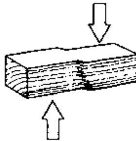
Vertical shear tends to deform wood cells perpendicular to their longitudinal axes. This type of shear is normally not considered for wood because other types of failures will occur before failure in vertical shear.
