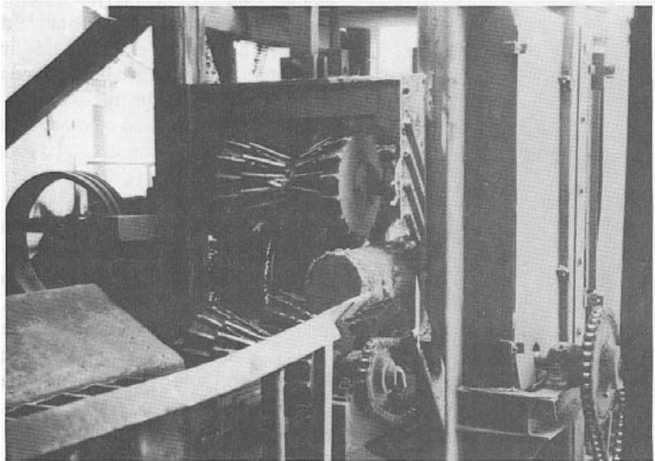
*Figure 4-3.- Removing bark is an important part of the treating process. In this photo, logs are debarked by rotating wheels prior to being sawn (photo courtesy of Kevin Rockwell, Southern Pine Inspection Bureau).*
