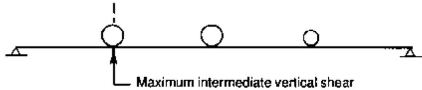
The maximum intermediate vertical shear for lane loads is produced by using a discontinuous uniform load with the concentrated load for shear ( $P_v$ ) positioned at the point where shear is computed.
