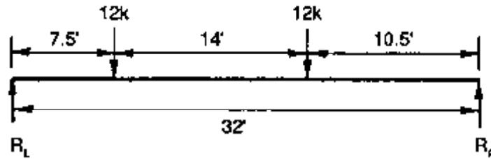
$$V_{LV} = R_L = \frac{(17.5 \text{ ft})(24 \text{ k})}{32 \text{ ft}} = 13.13 \text{ k}$$
