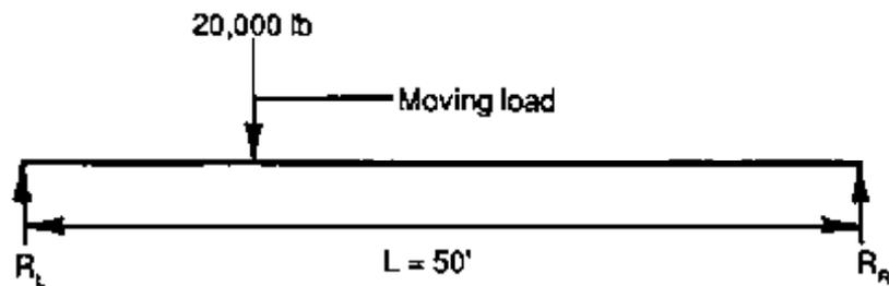
Case A: Lateral support is provided at beam ends and at third points
