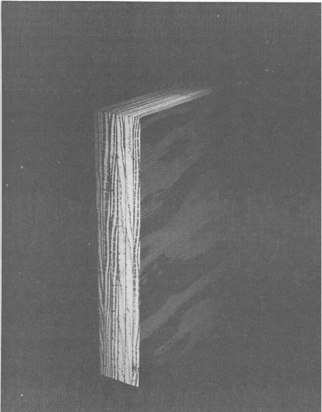
*Figure 2-8.- End section of an LVL beam; LVL beams are manufactured by gluing together sheets of veneer. The grain direction of the veneer layers is oriented in the same direction, parallel to the direction of the beam span.*
