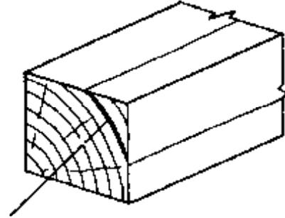
A shake is a separation or plane of weakness between growth increments that may extend a substantial distance in the longitudinal direction.
