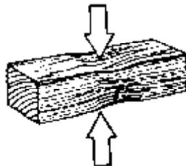
Compression perpendicular to grain compresses the wood cells perpendicular to their longitudinal axes.
