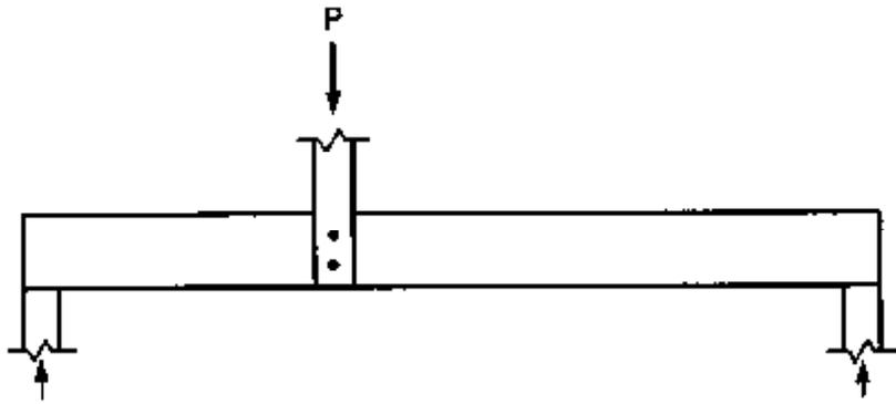
Figure 5-18. - Unsupported fastener loads applied transverse to the beam axis can reduce beam capacity in horizontal shear. Refer to the NDS<sup>26</sup> for design requirements for this loading condition.
