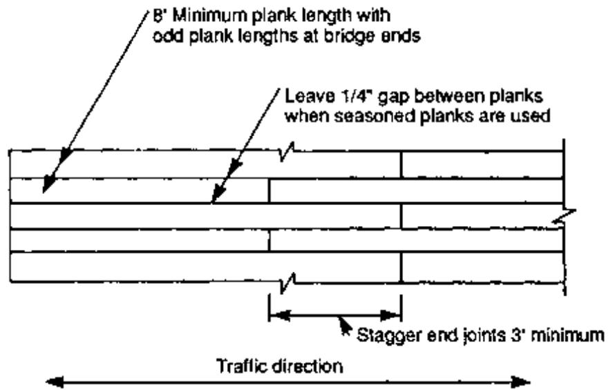
Figure 11-14. - Typical plank layout for lumber wearing surfaces.
