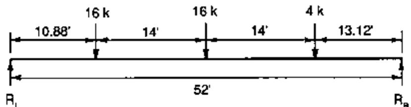
$$V_{LV} = R_L = \frac{(13.12)(4\text{k}) + (27.12)(16\text{k}) + (41.12)(16\text{k})}{52} = 22.01 \text{ k}$$
