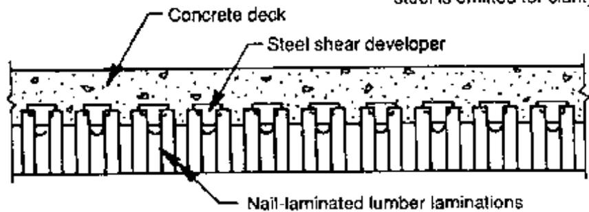
**Composite timber-concrete slab**
