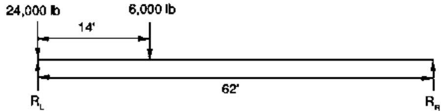
$$R_{MAX} = R_L = \frac{(6,000 \text{ lb})(62 \text{ ft} - 14 \text{ ft}) + (24,000 \text{ lb})(62 \text{ ft})}{62 \text{ ft}} = 28,645 \text{ lb}$$
