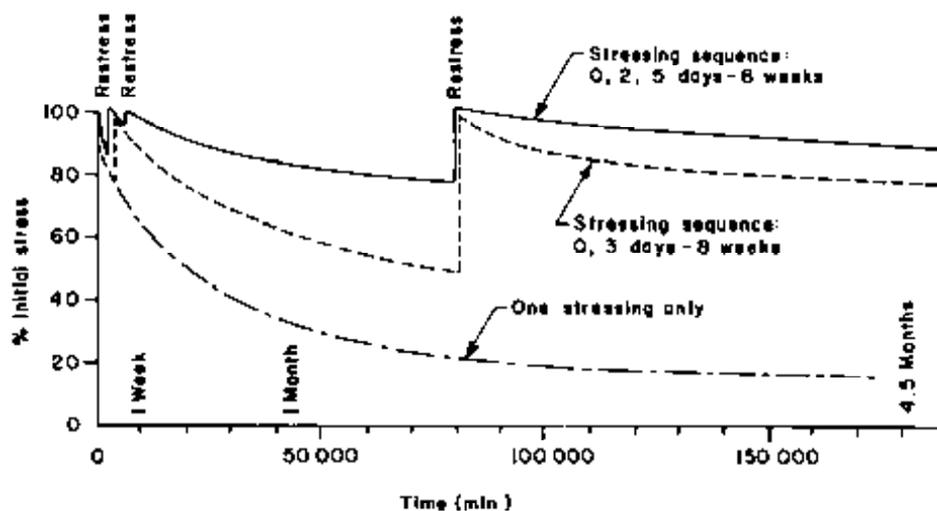
Figure 9-11. - Effects of restressing on time-related stress loss (from Csagoly and Taylor).<sup>8</sup>
