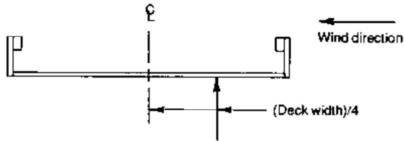
Upward wind force equal to 20 lb/ft<sup>2</sup> of deck and sidewalk area, applied at the windward 1/4 point of the deck width
