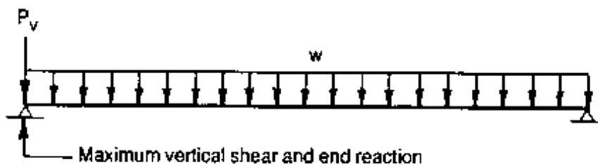
Maximum end reactions computed by these procedures are based on the bridge span measured center to center of bearings and are commonly tabulated in bridge design specifications and handbooks. Although they are technically correct for point bearing at span ends only, they do provide a very close approximation of the actual reaction for short bearing lengths. For very long bearing lengths, reactions should be computed based on the out-to-out span length with loads placed at the span end.
