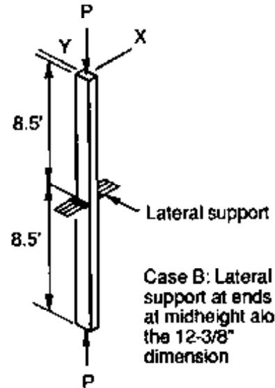
From Table 16-4, the area of an 8-1/2-inch by 12-3/8-inch glulam column is 105.2 in<sup>2</sup>.
