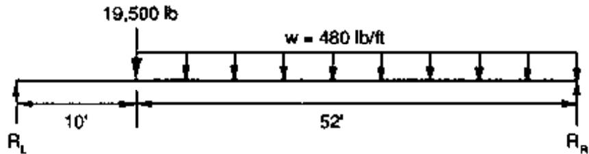
$$V_{MAX} = R_L = \frac{(480 \text{ lb/ft})(52 \text{ ft})(52 \text{ ft}/2) + (19,500 \text{ lb})(52 \text{ ft})}{62} = 26,822 \text{ lb}$$
