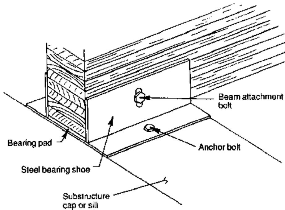
Figure 7-14. - Typical fixed-bearing configuration for glulam beams.
