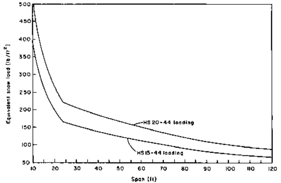
Figure 6-20. - Equivalent snow load required to produce the same moment as one truck load.
