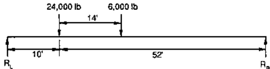
$$V_{MAX} = R_L = \frac{(6,000 \text{ lb})(52 \text{ ft} - 14 \text{ ft}) + (24,000 \text{ lb})(52 \text{ ft})}{62 \text{ ft}} = 23,806 \text{ lb}$$
