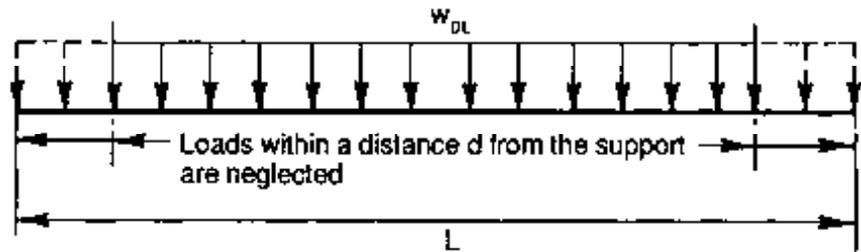
$$V_{DL} = w_{DL} \left( \frac{L}{2} - d \right) \quad (7-6)$$
