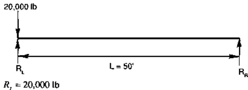
The reaction from the beam weight is the same at both supports:
