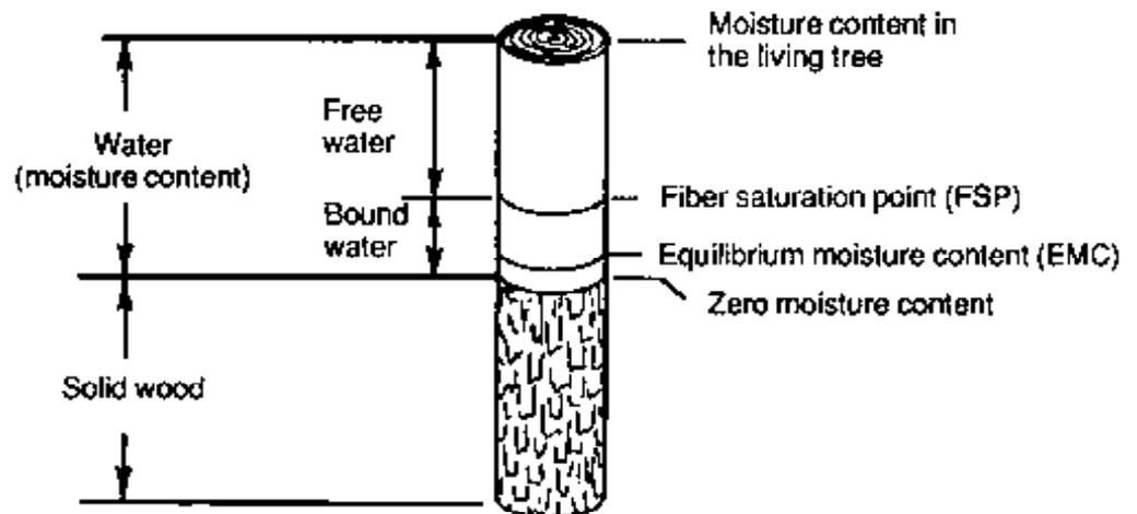
Figure 3-6.- Diagrammatic representation of wood moisture content.
