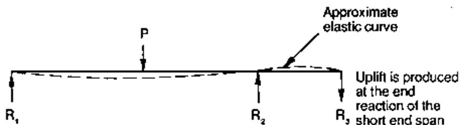
Figure 6-21. - Uplift force on a continuous-span superstructure.
