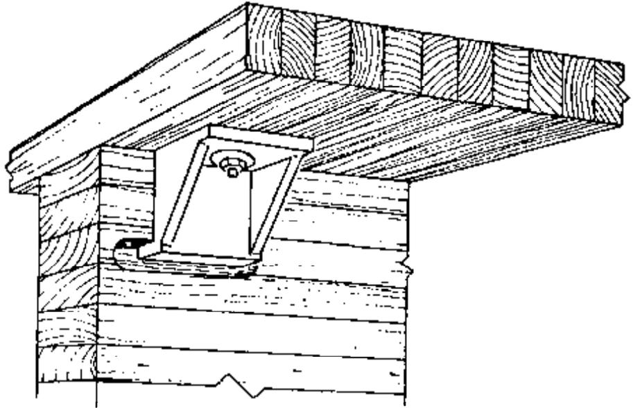
Figure 7-24. - Aluminum deck bracket for attaching glulam decks to glulam beams.
