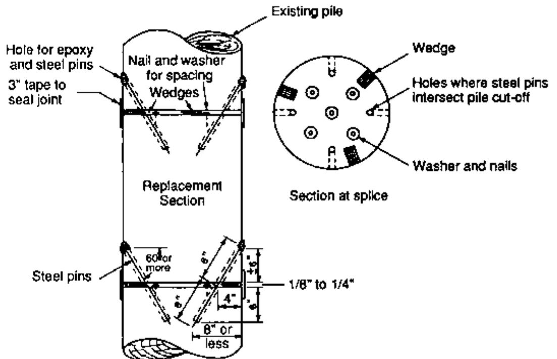
Figure 14-16. - Schematic diagram of pile posting.
