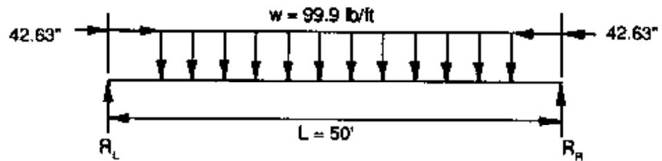
$$V = R_L = w \left( \frac{L}{2} - d \right) = 99.9 \left[ \frac{50}{2} - \frac{42.63}{12 \text{ in/ft}} \right] = 2,143 \text{ lb}$$
