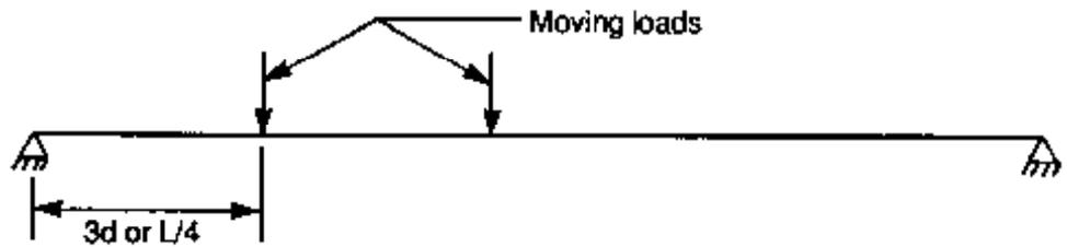
For moving loads, the loads are positioned to produce the maximum vertical shear at the lesser of 3d or L/4 from the support
