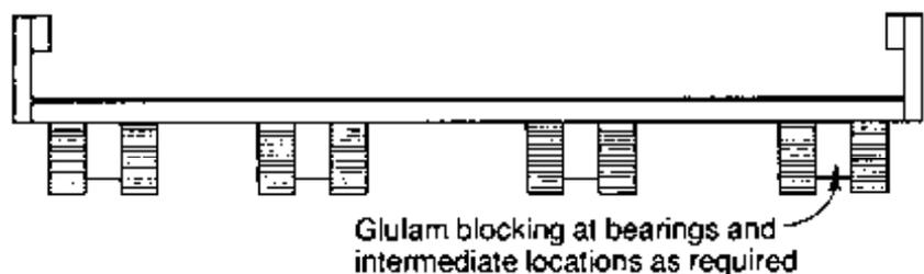
Figure 7-7. - Typical low-profile glulam beam configuration.
