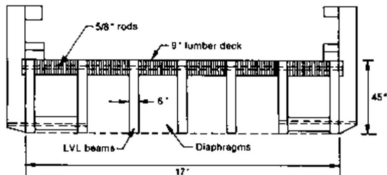
Figure 9-7. - Drawing of a stress-laminated T-bridge cross section.
