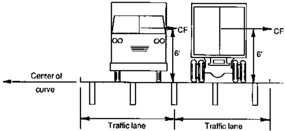
Figure 6-13. - Application of the vehicle centrifugal force.
