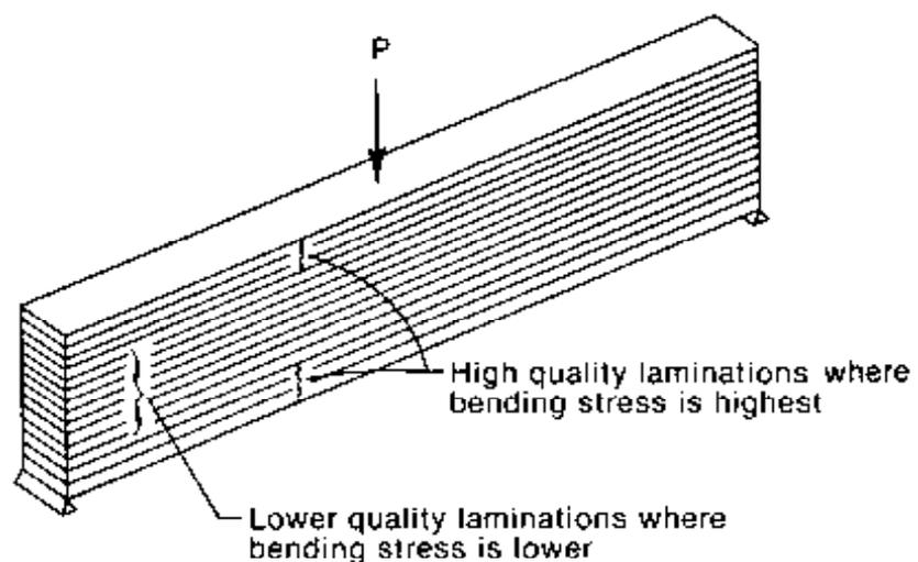
*Figure 3-33.-Glulam bending combinations are intended primarily for applications where loads are applied perpendicular to the wide face of the laminations. The quality of the lumber laminations is varied over the member cross section to provide higher strength where bending stress is highest.*
