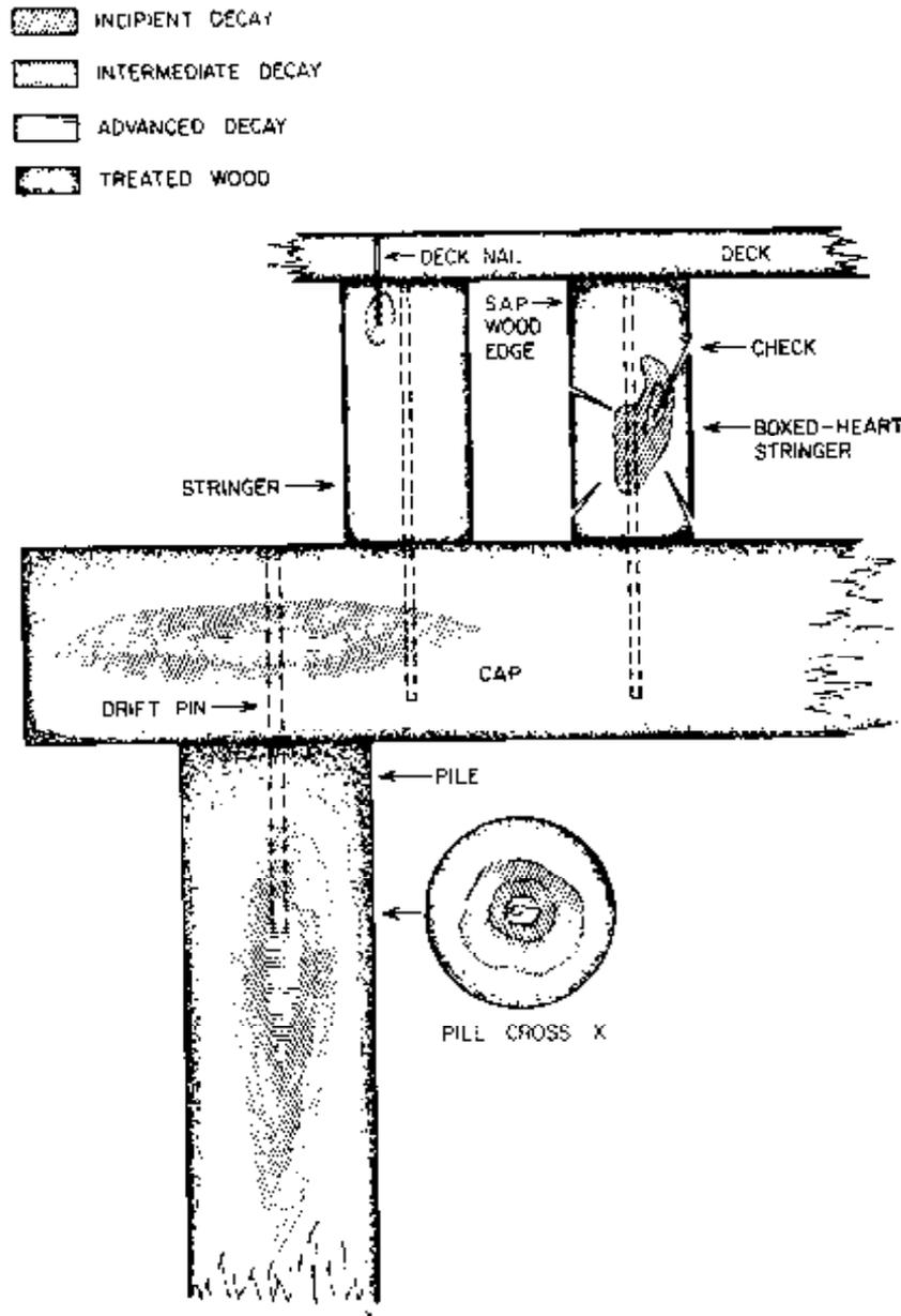
Figure 13-36. - Diagram depicting potential decay locations in a timber bridge.
