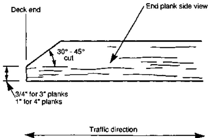
Figure 11-15. - Beveled end-plank configuration to minimize vehicle impact at bridge ends.
