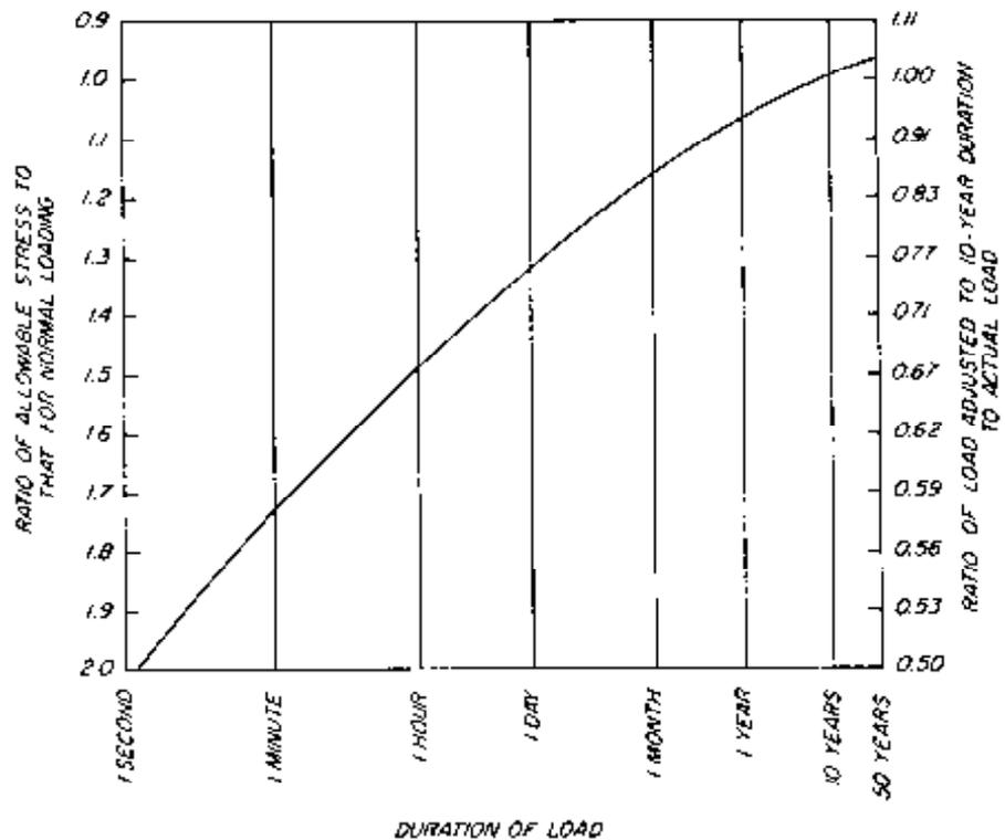
Figure 3-23.- Duration of load adjustment curve for wood.
