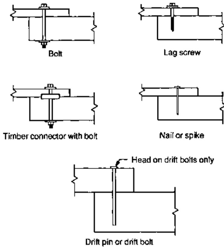
Figure 5-13. - Types of fasteners used for timber bridges.
