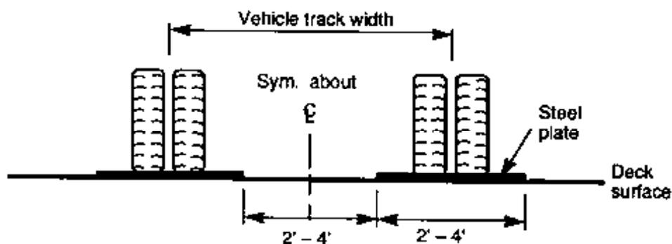
Figure 11-22. - Typical steel plate wearing surface cross section.
