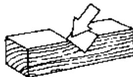
Compression at an angle to grain results in compression acting both parallel and perpendicular to grain.
