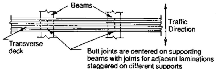
Figure 7-36. - Joint placement for transverse nail-laminated lumber decks.
