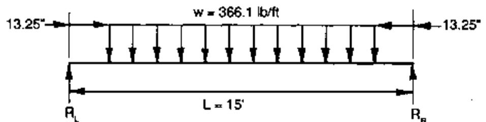
$$V = R_L = w \left( \frac{L}{2} - d \right) = 366.1 \left[ \frac{15}{2} - \frac{13.25}{(12 \text{ in/ft})} \right] = 2,342 \text{ lb}$$
