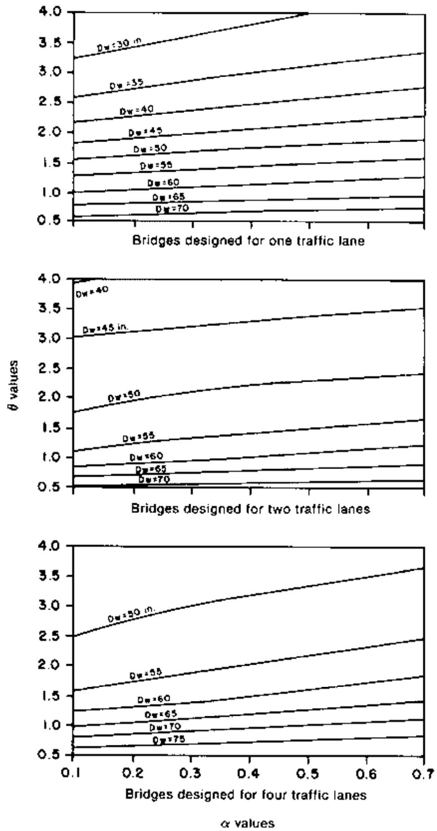
Figure 9-15. - Graphs for determining the wheel load distribution width ( $D_w$ ) for longitudinal stress-laminated bridge decks.
