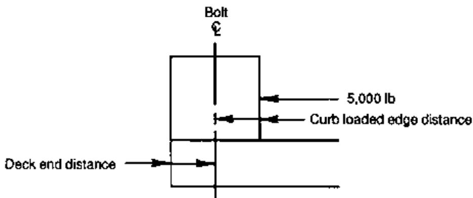
From Table 5-22, the minimum loaded edge distance for loading perpendicular to grain is four times the bolt diameter,
