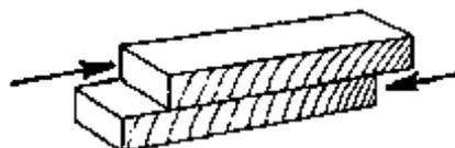
Rolling shear produces a tendency for the wood cells to roll over one another, transverse to their longitudinal axes. This type of shear is normally not a consideration for solid or laminated
