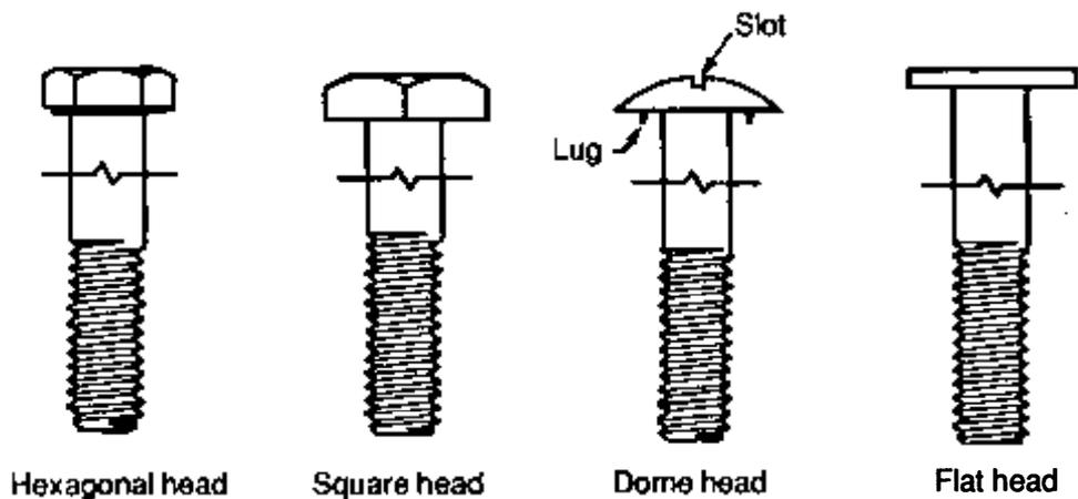
Figure 5-19.- Bolt types used for timber connections.
