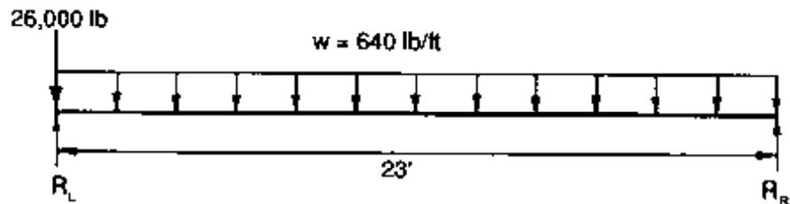
$$R_{MAX} = R_L = \frac{(640 \text{ lb/ft})(23 \text{ ft})}{2} + 26,000 \text{ lb} = 33,360 \text{ lb}$$
