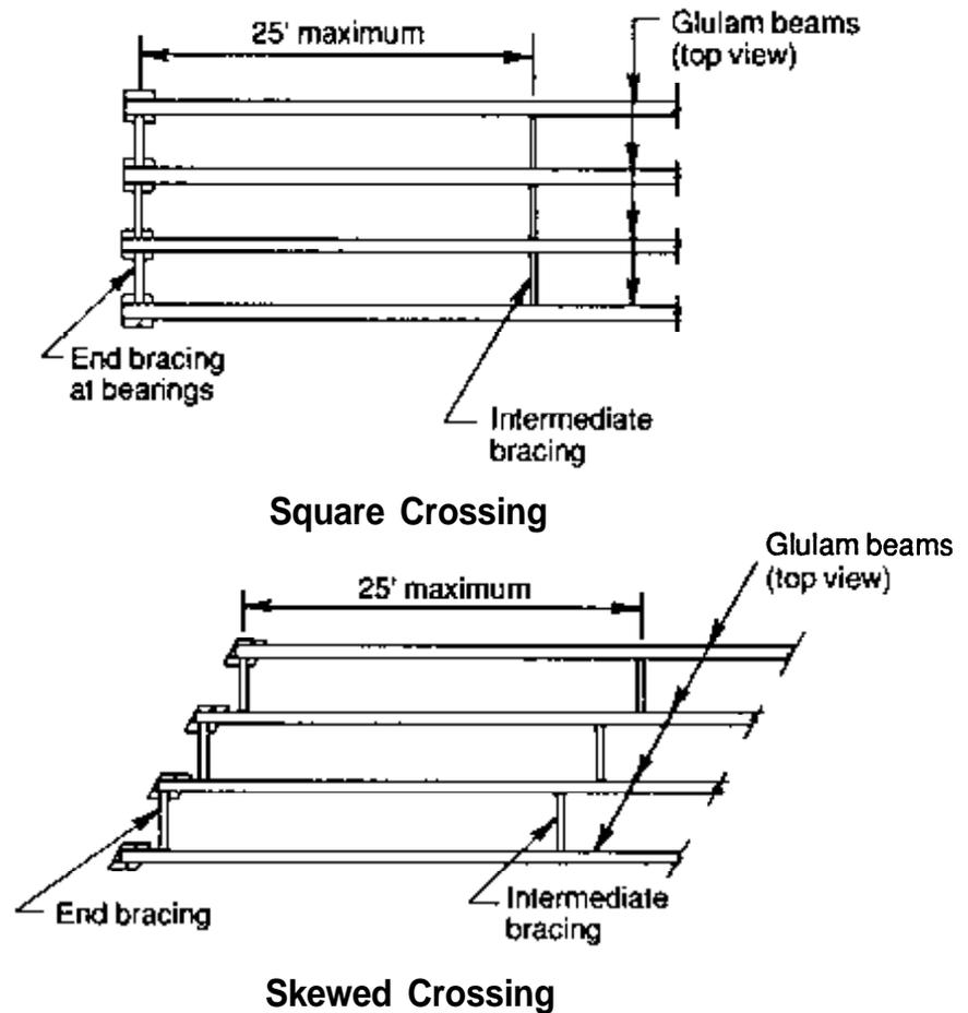
Figure 7-11. - Transverse bracing configurations for glulam beams.
