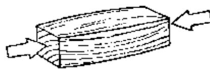
Compression parallel to grain tends to shorten wood cells along their longitudinal axes.
