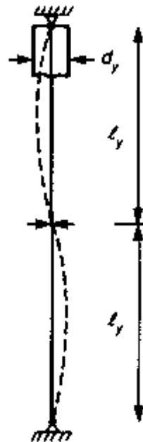
Buckling mode about the y-y axis  $(\ell_e/d)_y$
