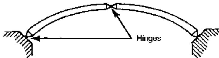
Three-hinge arch is hinged at reactions and at the arch apex.
