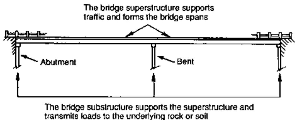
*Figure 2-1.- Basic components of a timber bridge.*
