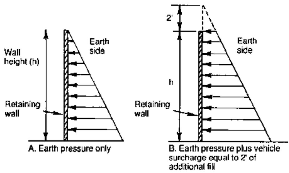
Figure 6-23. - Distribution of earth pressure on retaining structures.
